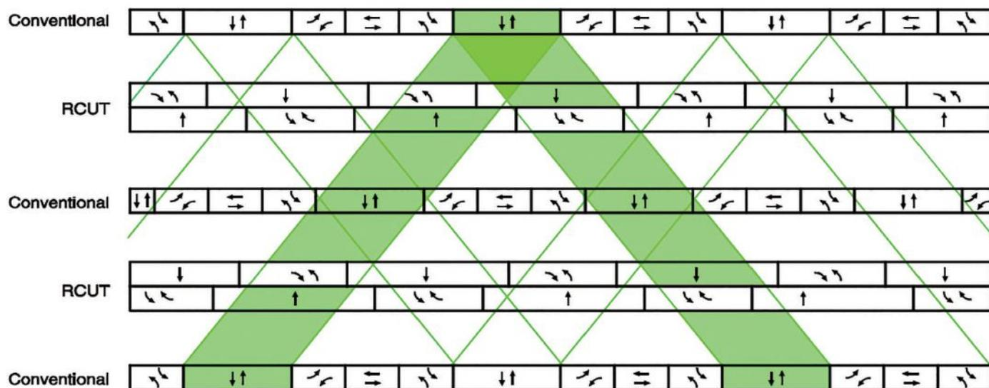
Figure 3: Example of two-way progression on an arterial with RCUTs and conventional intersections<sup>7</sup>
