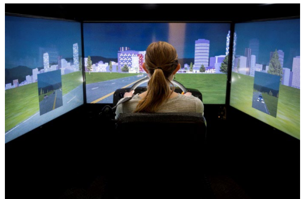
Figure 4: Quarter Cab Heavy Vehicle Driving Simulator
