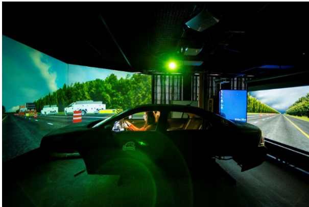
Figure 2: Full Cab Passenger Car Driving Simulator
