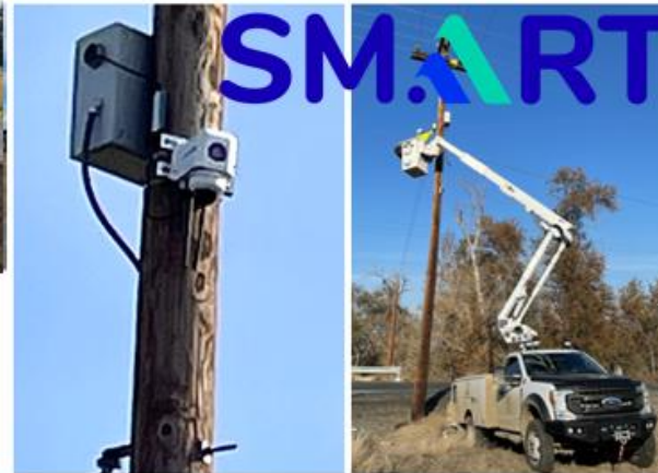
Edge AI Device for Traffic & Road Conditions Monitoring and Hazardous Events Detection
