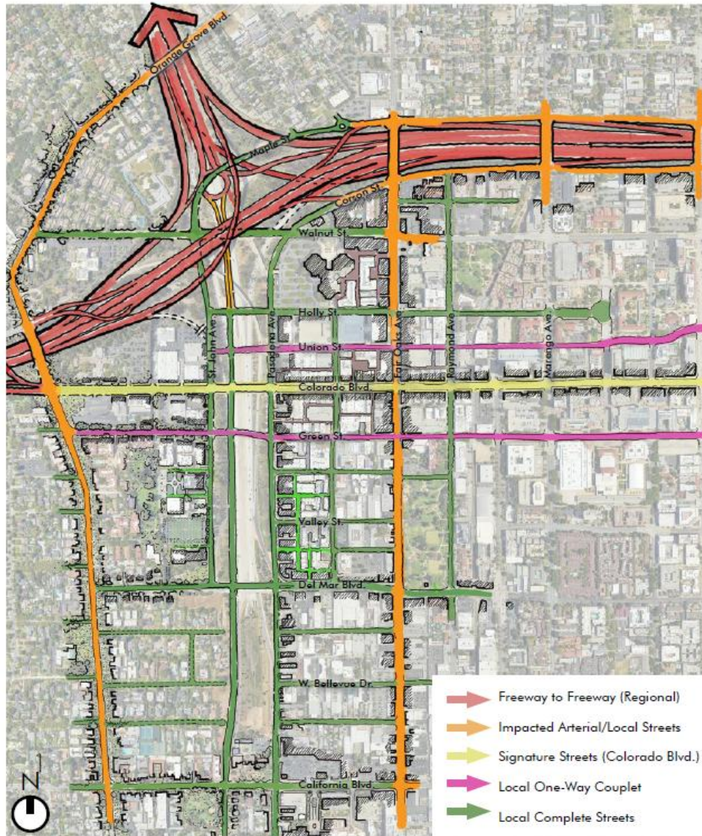
FIGURE 4.7: ONE OF THE OPTIONS FOR A STREET NETWORK AND STREET CLASSIFICATIONS, SHOWING A SHIFT TOWARDS MORE LOCAL CONNECTIONS. THIS FIGURE SHOWS THE "BOULEVARD AND PASEOS" CIRCULATION NETWORK FOR PURPOSES OF ILLUSTRATION. THE DIAGRAM REMOVES THE REGIONAL LINKS AND REPLACES THEM WITH THREE SURFACE LEVEL STREETS (SHOWN IN GREEN).
