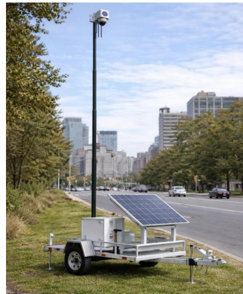
Solar-powered trailer-mounted deployment
