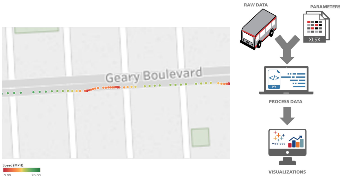
Figure 2a (left): Illustration of location data for a single trip approaching a far-side bus stop at Geary Boulevard & 9 th Avenue and subsequently stopping at the following signalized intersection.
