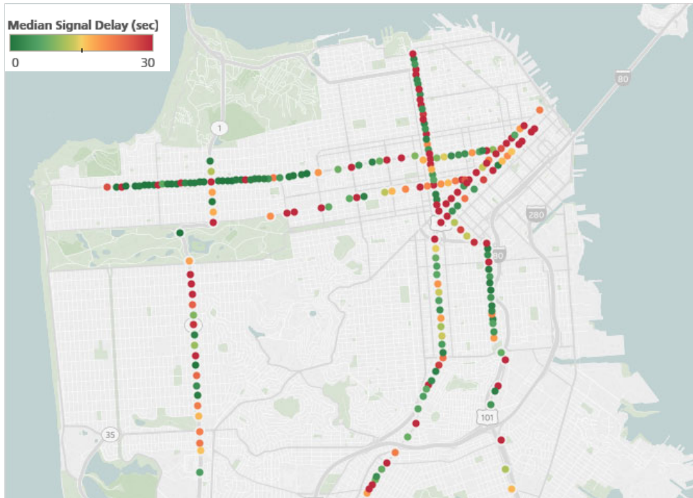
Figure 3: Visualization of median signal delay across a subset of the SFMTA system focused primarily on Rapid and frequent corridors.
