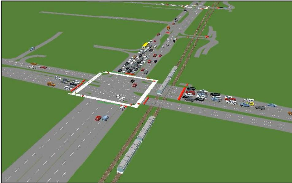
*This screenshot, captured during a simulation run of the Area B PM Peak Vissim model, shows two trains crossing Alameda Avenue in parallel with the vehicles on northbound and southbound Sable Avenue. The linked crossings at the Commercial Access and Bayaud Avenue are visible in the background.*
