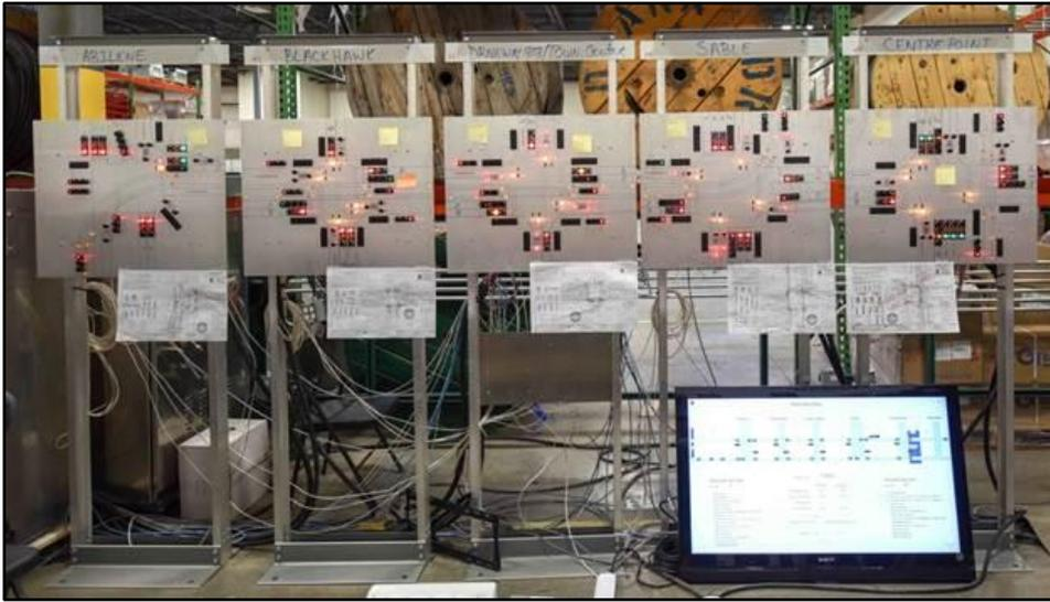
*The first part of bench testing for Area B focused on the five crossings between the Florida and Aurora Metro Center stations. The light boards for each crossing are each hooked up to a separate signal controller, while the screen at the bottom displays the status of trains during each test.*
