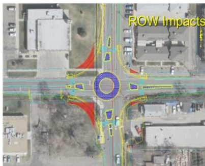
Right-of Way Requirements at the Intersection
