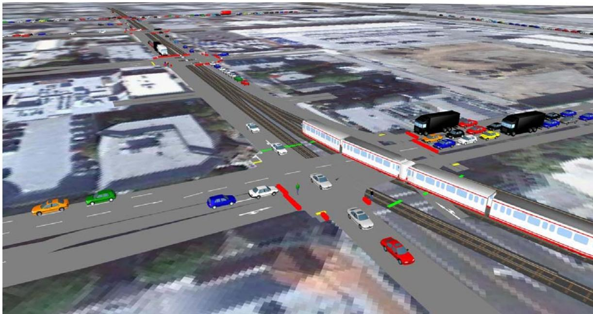
Traffic operation analyses were conducted for the peak hours. Measures of effectiveness such level of service, intersection queue and travel time were obtained from VISSIM model output. These measures of effectiveness were used to compare alternatives and to analyze the impact of the LRT alignment on the traffic operations.
