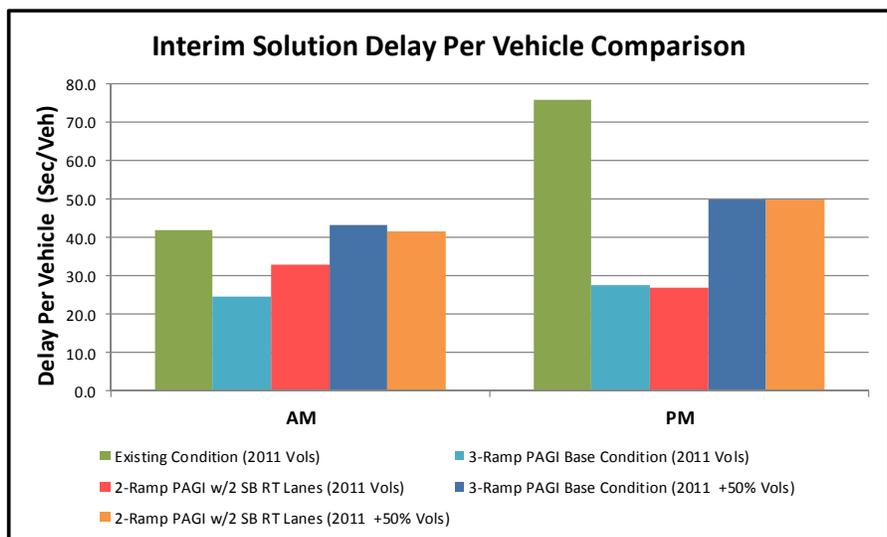
volumes of left-turns can be accommodated by coordinating the downstream left-turn green with the upstream main intersection.
