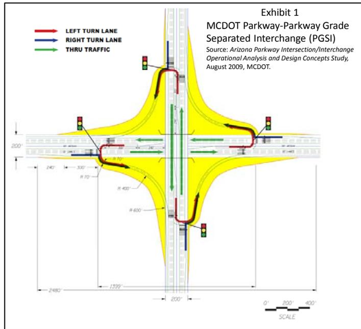
The PGSI became the origin of the new PAGI at-grade intersection concept where the main intersection is also controlled by a simple 2-phase traffic signal. The flexibility of the ramp design and placement, and the overall capacity of the concept exceeded the requirements for the Pima County application.
