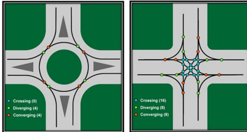
Figure 1. Conflict Points at Roundabout vs. Intersection (Source: FHWA)
