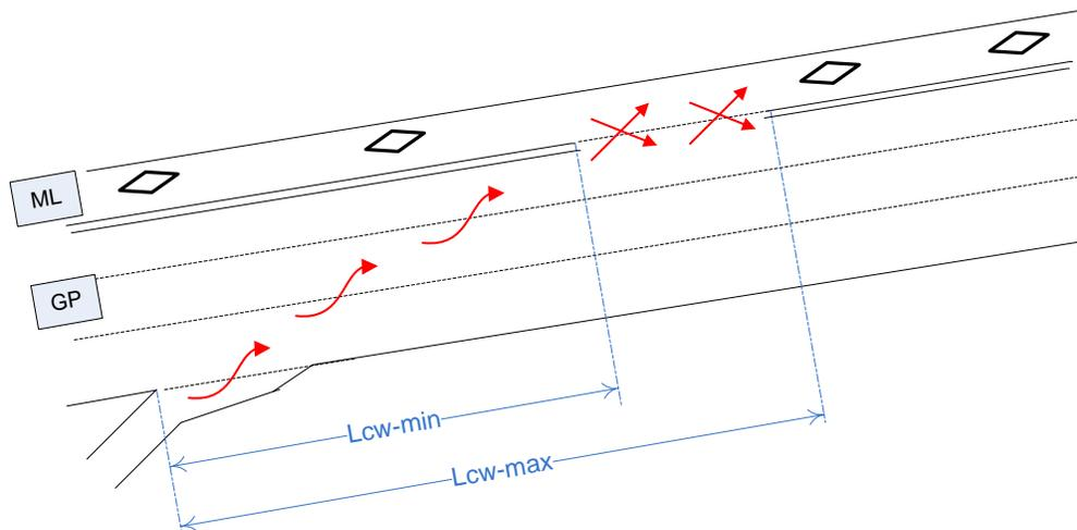
**FIGURE 3: Defining Dimensions of APIA through Minimum and Maximum Cross-Weave Lengths**
