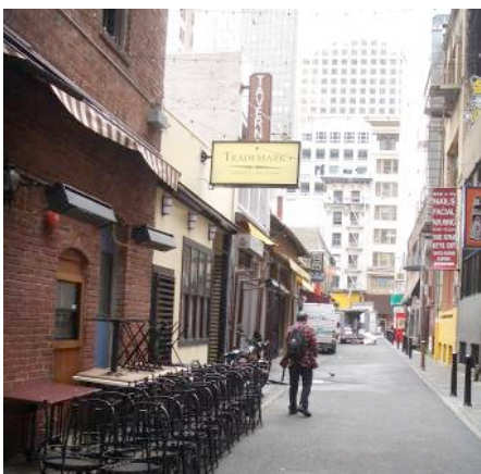
Figure 2 (above): Belden Place in San Francisco's financial district is an alleyway that allows for deliveries but also serves as a safe pedestrian environment with a variety of restaurants and outdoor seating. The geometric design includes a single-plane surface.
