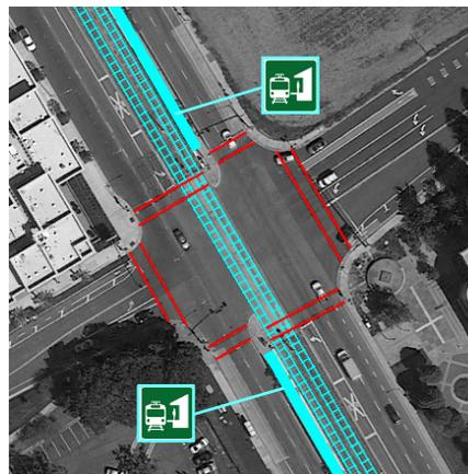
Median-running light rail transit (LRT) station adjacent to intersection with TSP
