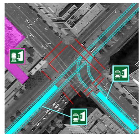
Intermodal hub (HRT terminal with median-running LRT) adjacent to intersection with TSP
