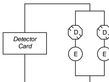
**Figure 4-3: Wiring Configuration Three**
