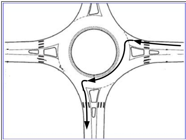
**Figure 1 Diagram showing a vehicle making an illegal left-turn at a roundabout**
