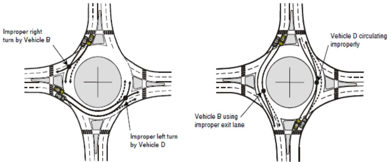
**Figure 3 Diagram showing improper lane use at two lane roundabouts**
