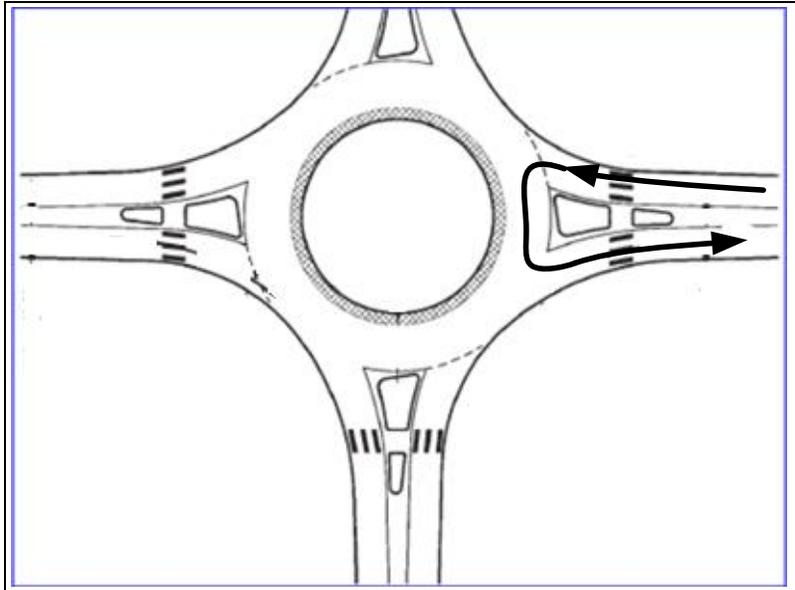
**Figure 2 Diagram showing a vehicle making a U-turn at a roundabout**
