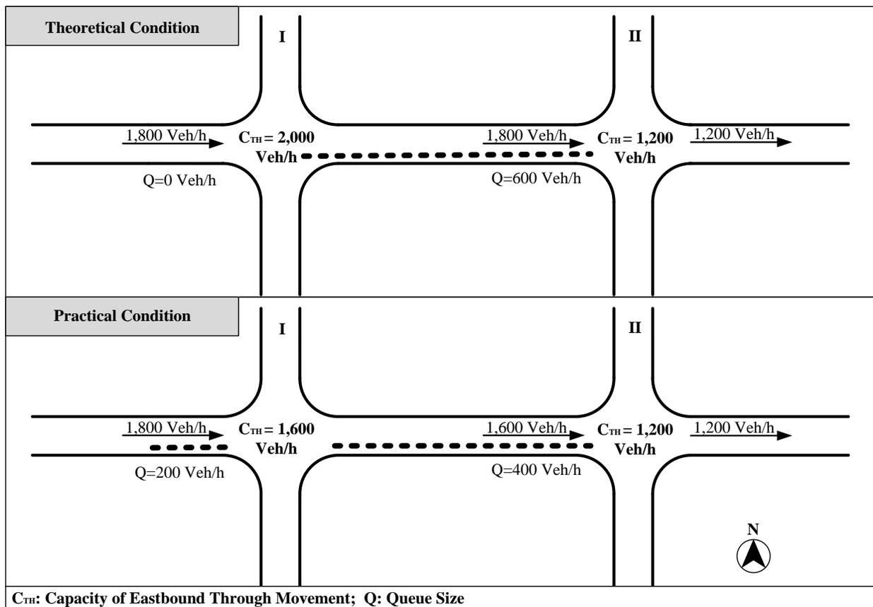
**Figure 1. Demonstration of Queue Spillback between Paired Intersections**
